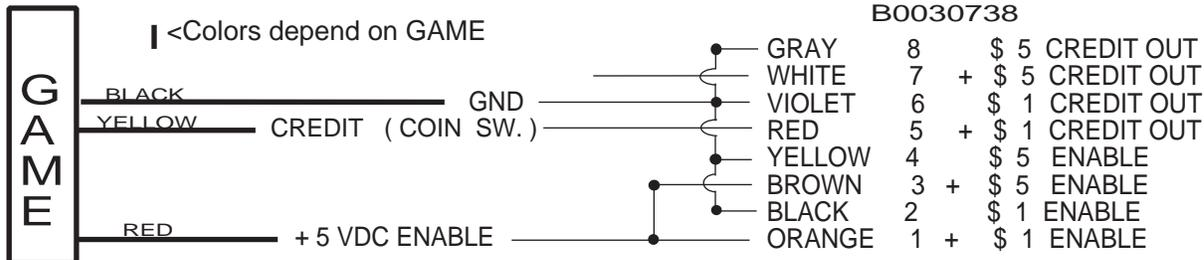
For any given interface for a CBA-2/UCBA-2 it is best to look at the manual. Interface. Switch settings vary a great deal. This interface is just one of many interfaces. This interface uses ROWE's 8 wire cable plugged into P3.
